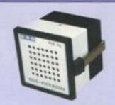
These are fully solid state device having long life & low power consumption. Generates no radiofrequency noise. Protected against polarity reversal. Suitable for panel cutout size 92x92 mm. Available voltages 12V, 24V, 110V, 220/230V DC/AC. Also available in multi tone version. Sound output 95 db to 100db.
