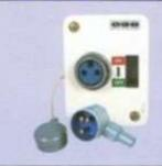
In locations where the atmosphere is corrosive and contains dust suitable enclosures are used. Effective protection to both against over load & short circuit should be provided by mounting suitably rated MCB. These boxes are wired from inside. Plugs & sockets are being tested in house as per IS/IEC 309 part 1 & 3.
